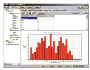
**Network Latency Measurement** In providing Voice over IP to remote telephones, considerations such as headquarters-to-branch latency and voice data bandwidth requirements must be taken into account. The MD1230A family can easily measure the end-to-end latency with microsecond precision and the transmission bandwidth between business centers and voice destinations for planning internal engineering support service criteria (such as VPN integrated services planning) and customer SLA development.
