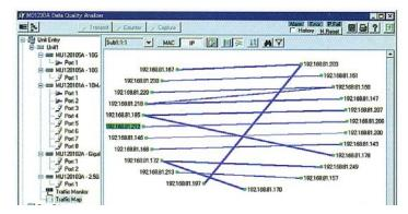
source/destination pairs by source and destination addresses. The Traffic Monitor real time display shows counts by Ethernet address, IP address, or protocol types for up to 64 communicating partners.
